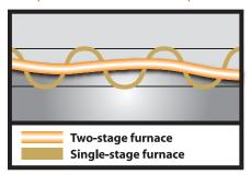
A two-stage furnace can operate at high or low output capacity to accurately and efficiently control home comfort in relation to outside temperature and home heating needs.
